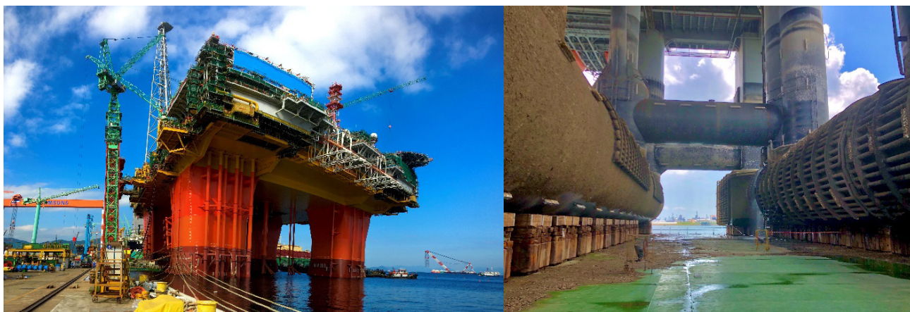
Figure 4. Mobile offshore drilling units (left) and other non-standard maritime platforms used in the offshore industry often have complex subsea niches (right) and can support diverse biofouling communities.
